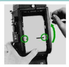
3. Pull out the leader paper of the film and insert it into the slit of the take-up spool, turn the film advance crank clockwise until the start mark on the leader paper matches the start marks on the camera.
